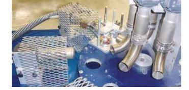
High-end air heaters on an indexing table for producing light bulbs.
